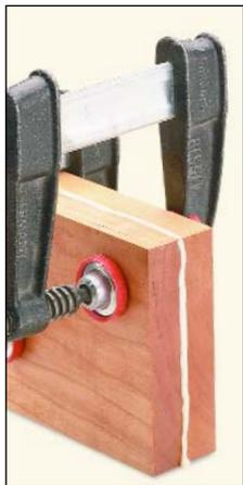
▲ Bracket feet look like they were cut from thick blocks of wood, but these blanks were made with two pieces of ¾"-thick stock.
