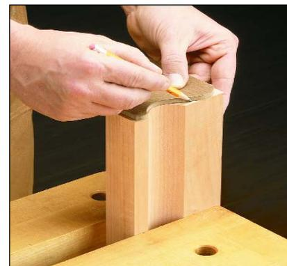
▲ Hardboard makes a good, reusable template for the bracket feet profiles, see pattern at left. To position the template on the blank, just line it up with the cove you've already cut.
